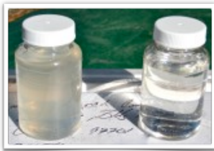
Septic tank effluent versus MBR effluent for a residential MBR system in Oregon
