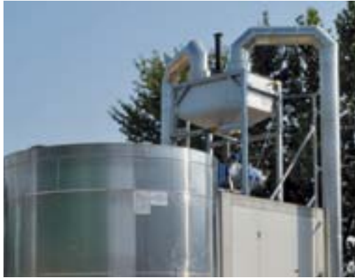
The fermenter separation guarantees a constant amount of dry matter.
